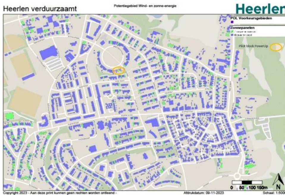
Figure 21 - Map of Vrieheide solar potential. In green: the properties on which solar panels have already been installed. In purple: properties with potential for solar panels as part of the pilot. The circled location is where the pilot will run.
